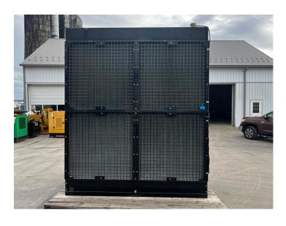
CAT RADIATOR/COOLING PACKAGE, UNUSED SURPLUS, TO FIT 3516B, DUAL CIRCUIT JACKET WATER AND AFTER COOLING
