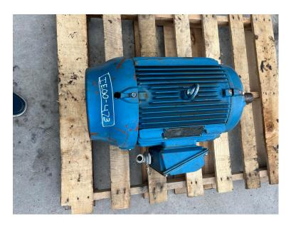
WEG ELECTRIC INVERTER DUTY, SEVERE DUTY, 3 PHASE, AC MOTOR, 20 HP, WITH 1 7/8" SHAFT, 1175 RPM, GOOD USED, TESTED
