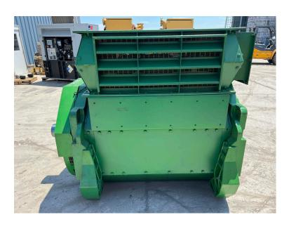
STAMFORD JENBACHER REBUILD GEN END, 2400 KW, 2 BEARING, CONTINUOUS DUTY, 480 VOLT, 1800 RPM
