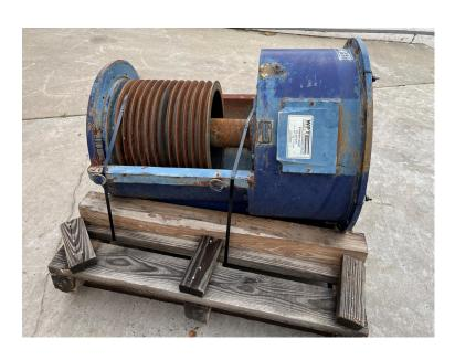
PTO CLUTCH FOR INDUSTRIAL ENGINE UP TO 1000 HP W/
