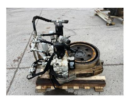
HYDRAULIC DRIVE ADAPTOR WITH SAE 0, 18 IN. IND. INPUT AND OUTPUT WITH 3 HEAVY HYDRAULIC PAD MOUNTS FOR HYDRAULIC PUMPS
