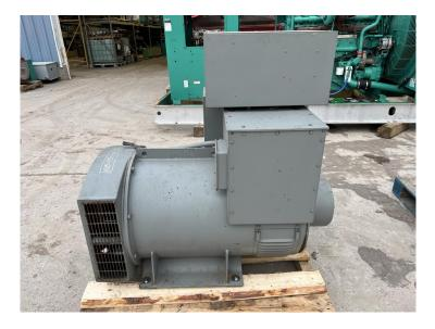
Voltage 277/480 Volts Hours 824 Hours Phase 3 Make Newage/Consolidated Power, Ind. Model 300D6T Serial W4305 Wires 10 Kilo Watts 300 kW Length 50" Width 37" Height 46" Weight 2500 lbs Condition Good Used Bell SAE 1 Flywheel 14" Ind.
