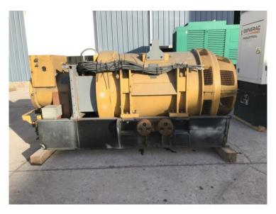
Year 2010 Hours About 1800 Hours Make CAT Model 1020FDS5716 Serial WA-574310-0910 Hertz 60 Hz Part 324-2355-00 Length 126" Width 66" Height 68" Weight 20,000 lbs Condition Well Maint. Unit, Tested, Serviced, Ready to go! Bell SAE 00 Flywheel To Fit C175 CAT
