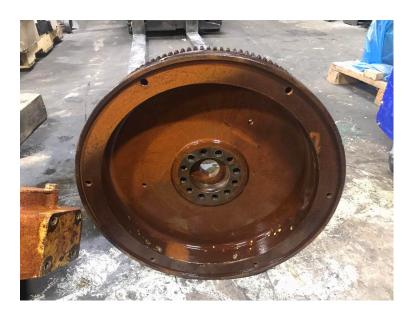
CAT ENGINE FLYWHEEL TO FIT INDUSTRIAL SAE 0 HOUSING + 18 INCH INDUTRIAL CLUTCH OR GEN. TO FIT CAT 3406 C15 C18 3408 3412 C32 C27 ENGINE MODELS
