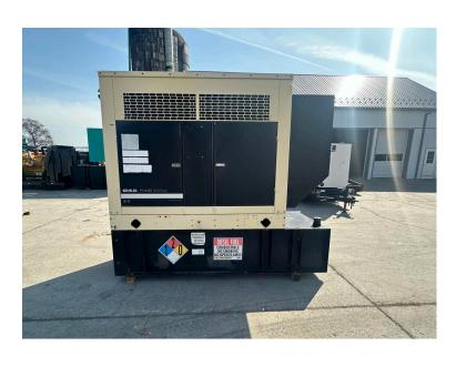
\_\_80 KW KOHLER GENSET WITH SOUND ATTENUATED ENCLOSURE AND BASE TANK, 4.5 JOHN DEERE ENGINE, YEAR -2003
