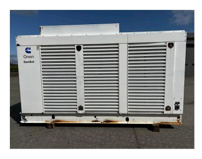
\_500 KW CUMMINS/ONAN KTA19G4 GENSET, WITH ENCLOSURE, YEAR - 1996, 416 HOURS
