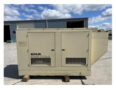
Fuel Diesel Year 2004 Voltage 120/208 Volts Hours 2038 Hours Phase 3 Phase Make Kohler Model 30RE0ZJB Serial 0795136 Hertz 60 Hz Wires 12 Lead Kilo Watts 33 kW Mounted Skid Mounted Enclosed Enclosed Lead Reconnectable Length 120" Width 45" Height 70" Weight 3500 lbs Condition Well Maint. Unit, Tested, Serviced, Ready to go Circuit Breaker Yes
