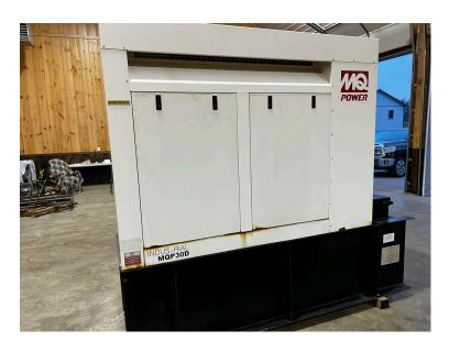
\_30 KW MULTIQUIP GENERATOR, ENCLOSED, BASE FUEL TANK, DEUTZ ENGINE, YEAR - 2007
