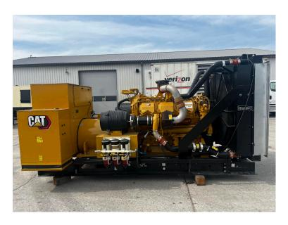
1000 KW CAT GEN SET, C32, US EPA TIER 2 PRE EMISSION ENGINE, OPEN SKID, YEAR -2021, 25 HOURS SINCE NEW
