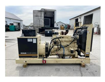
\_100 KW KOHLER DIESEL GENSET, JOHN DEERE ENGINE, YEAR 1999, 659 HOURS, 120/240 VOLTS, RECONNECTABLE
