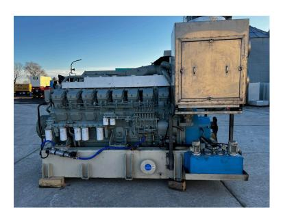
S16R MITSUBISHI DIESEL ENGINE WITH LESS THAN 500 HOURS SINCE NEW. TAKEN OUT OF A DATA CENTER, BACKUP GENERATOR, US EPA TIER 2 PRE EMISSIONS, YEAR - 2014
