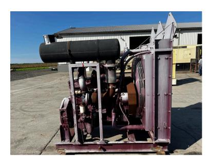
QSM11 CUMMINS INDUSTRIAL POWER UNIT ENGINE, 375 TO 400 HP, YEAR - 2010, US EPA TIER 3, PRE EMMISSIONS ENGINE
